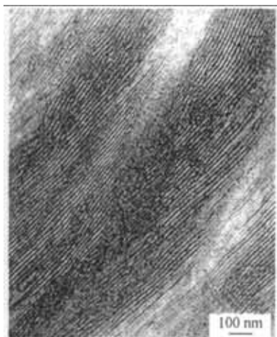
Fig. 12 TEM observation of the lamellar morphology of an ultramicrotomed EOS-L thin film sectioned along the thickness direction after staining by RuO 4
